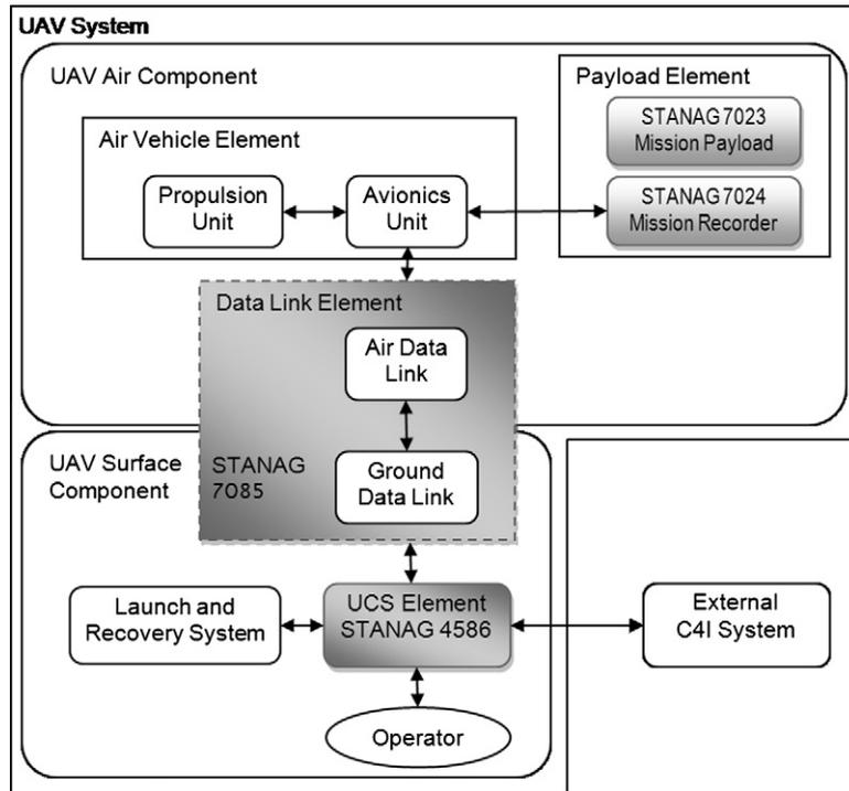
Fig. 5. UAV system interoperability architecture with STANAG 4586.
